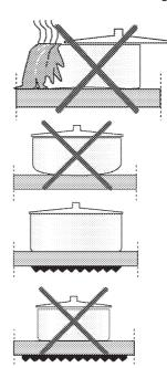
Spills may damage the glass ceramic surface and cause fire.
